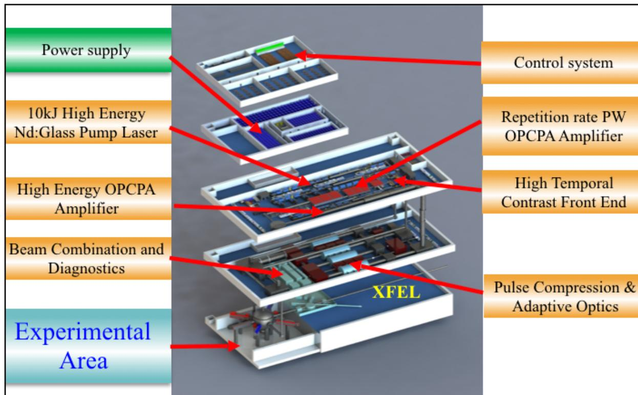
Schematic layout of the 100 PW laser system at the Station of Extreme Light of the proposed Shanghai Coherent Light Facility.
