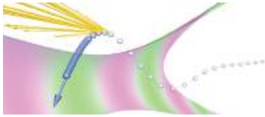
Fig. 1. An electron (blue) oscillates under the action of strong laser fields (green/purple), emitting energetic bursts of \gamma rays (yellow). The recoil of this emission causes the electron to slow down.
