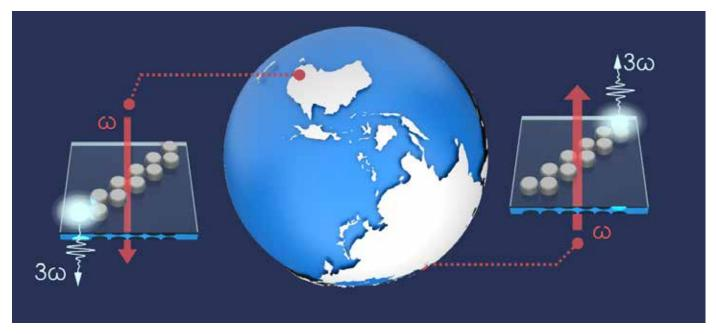
Concept of nonlinear parametric topological edge states as seen from Canberra and from Moscow perspective. Third-harmonic generation from edge states in a zigzag array of silicon nanoresonators depends on the pump direction.
