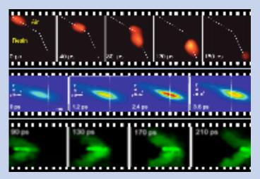
Fig. 1. World's fastest camera captures light refraction (top row), temporal focusing (middle row), and propagation of photonic Mach cone (bottom row) in real time. [Nature 516, 74 (2014), Light: Sci. & Appl. 7, 42 (2018), and Sci. Adv. 3, e1601814 (2017
