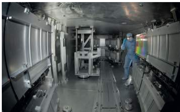
Engineer JB McLeod inspects one of the first four high-efficiency diffraction gratings installed in the ARC compressor vessels. ARC's one-meter-wide multilayer dielectric gratings were specially developed at LLNL to withstand the record levels of energy generated by NIF's lasers.
