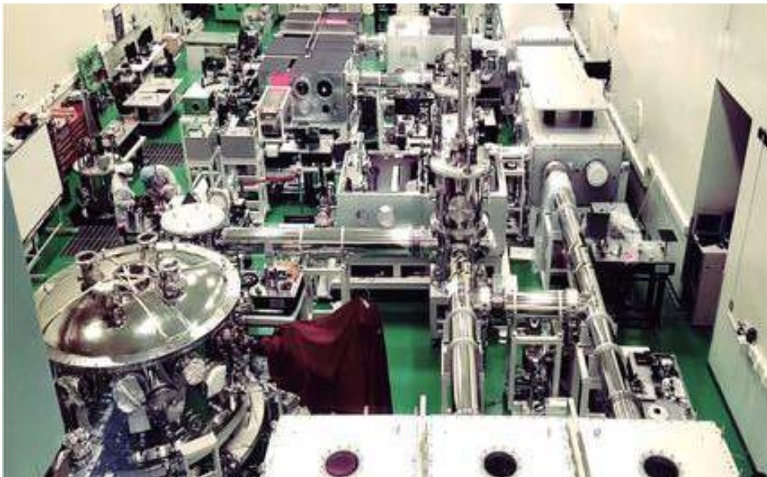
Fig. 2. Experimental area showing three target chambers and a double plasma mirror chamber along with two pulse compression chambers.
