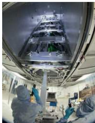
Technicians monitor the successful insertion of transport mirrors in the 11-foot-high ARC Parabola Vessel. The Parabola Vessel will focus ARC's quadrillion-watt beams on backlighter targets near Target Chamber center to produce an x-ray "movie" to diagnose NIF target implosions.
