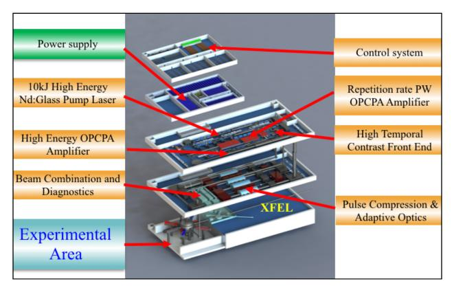
Schematic layout of the 100 PW laser system at the Station of Extreme Light of the proposed Shanghai Coherent Light Facility.
